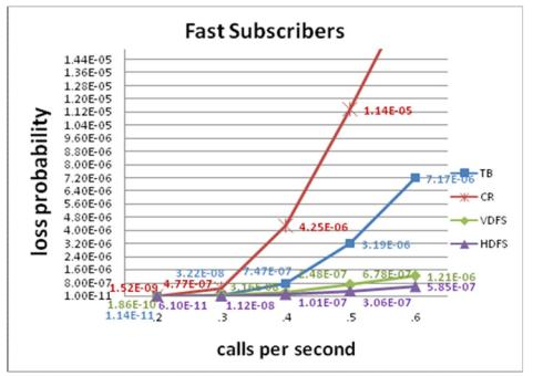
Figure 4(B): Numerical analysis comparison on call loss probability for fast subscribers
