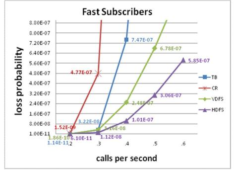
Figure 4 (A): Numerical analysis comparison on call loss probability for fast subscribers
