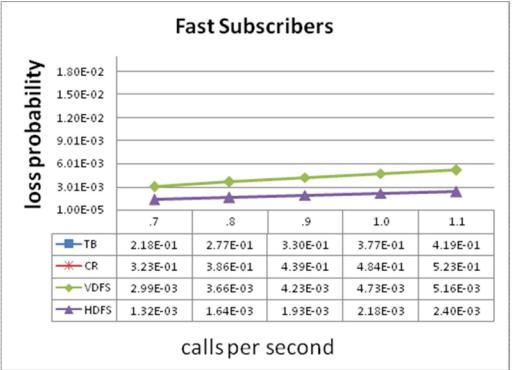
Figure 6(B): Numerical analysis comparison on call loss probability for fast subscribers (VDFS & HDFS)
