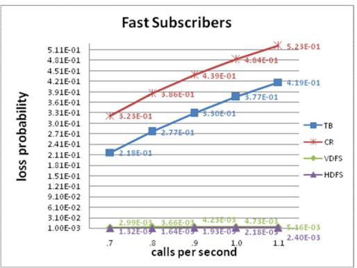
Figure 6(C): Numerical analysis comparison on call loss probability for fast subscribers
