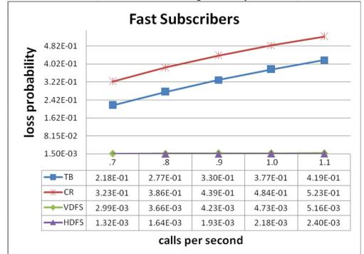
Figure 6(A): Numerical analysis comparison on call loss probability for fast subscribers (TB & CR)
