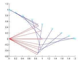
Figure 3. Moving trajectory of the manipulator using inverse kinematics.
