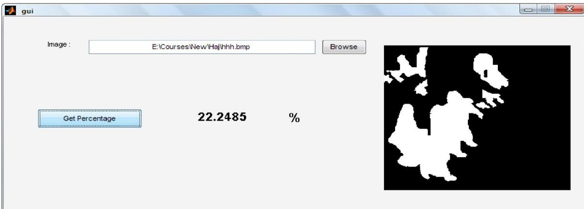
**Figure 10:** Density calculation using a thermal image without background.
