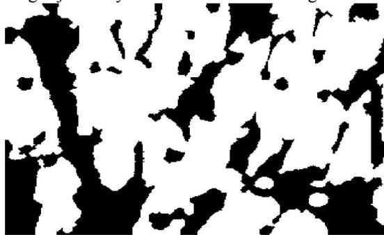
Figure 15: Binary image after subtracting background (Figure-14) from thermal image (Figure-12)
