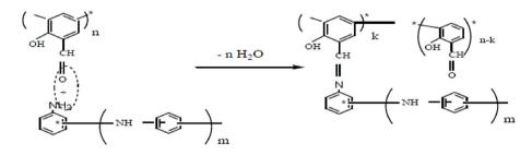
**Figure 9**. The preparation of graft-copolymer – copolyanilinehydroxybenzaldehyde (CAHB) has been carried out by joint condensation of oligoaniline(OA) & oligohydroxybenzaldehyde (OAHB) containing active amine & aldehyde groups respectively[13].
