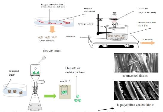
**Figure 13.** Coating processes of conducting polyaniline on to a flexible substrate such as textile fabrics & SEM observation of polyaniline coated fabrics (a,b) (SEM Figures from [16]).
