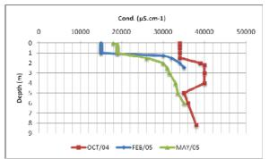
Figure 4. Electrical conductivity in the water columm during the period studied
