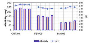
Figure 7. The relationship between pH and Alkalinity in water column during the period studied
