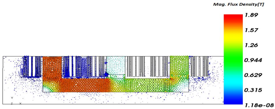
**Fig.1.9.** Flux Distribution with DC bias of 1A
