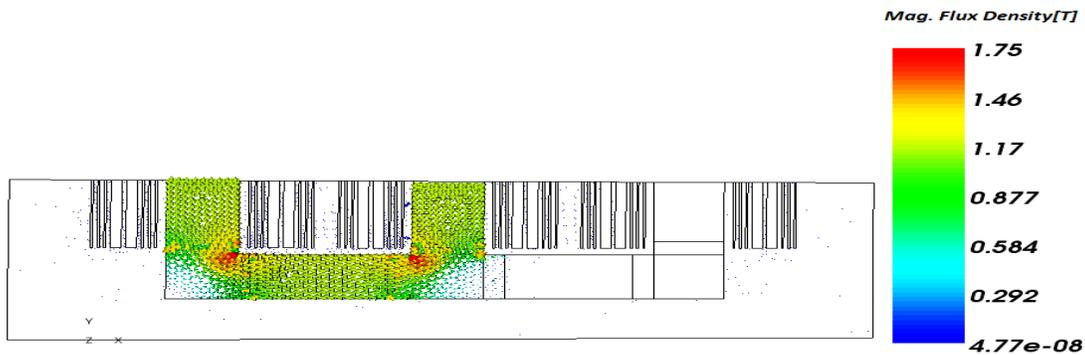
**Fig.1.7.** Flux Distribution in Transformer Without DC [Zero or 0] bias
