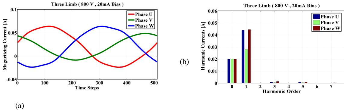
**Fig.1.4** (a) Magnetizing Currents (b) Harmonics at [Input Primary Voltage=800V, 20mA DC Bias]
