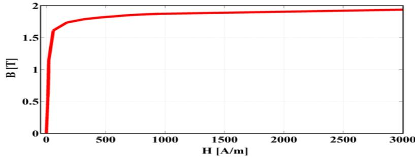
Fig.1.2. BH Curve for TKESC120 core material
