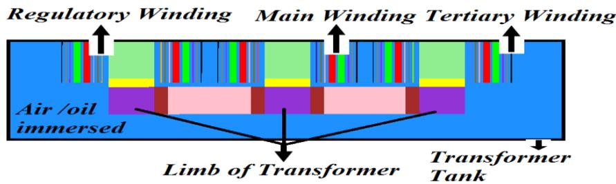
Fig.1.1. Two dimensional Three-Phase Three-Limb transformers FE Model
