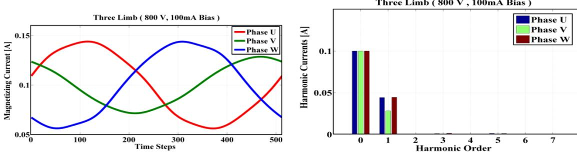
**Fig.1.5** (a) Magnetizing Currents (b) Harmonics at [Input Primary Voltage=800V, 100mA DC Bias]
