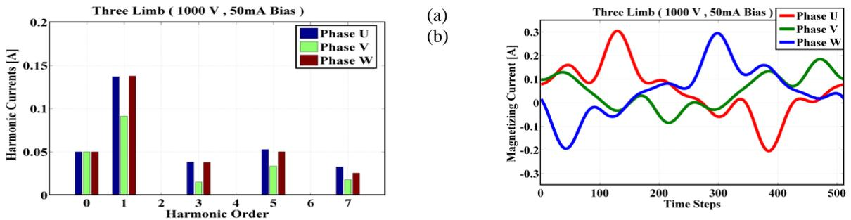
**Fig.1.6** (a) Magnetizing Currents (b) Harmonics at [Input Primary Voltage=1000V, 50mA DC Bias]
