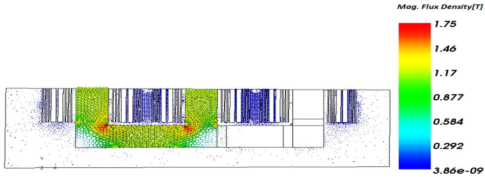
**Fig.1.8.** Flux Distribution in Transformer With 75mA bias
