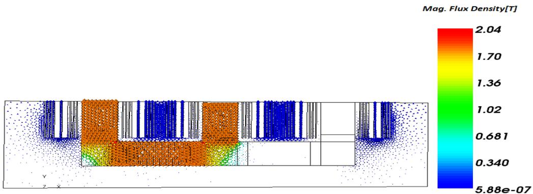
**Fig.1.10.** Flux Distribution with DC bias of 2A
