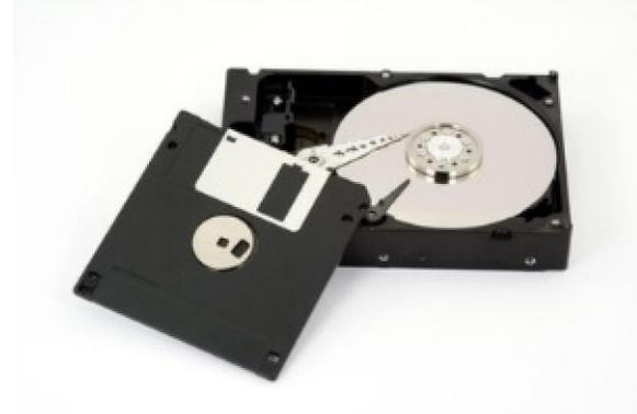
The original floppy disk was floppy and flimsy in texture. During the evolution of the floppy disk, they went from 80 kilobytes of storage up to 2880 kilobytes of storage (2.88 megabytes). The most known floppy drives are the 5 1/4-inch 720 kilobyte disk and the 3 1/2-inch 1.44 megabyte disk.
