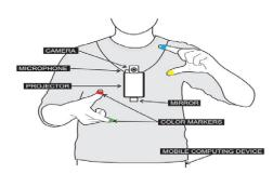
Now that you have all these pieces, you need a way to combine them. We recommend using Lego strips to form the base. The projector, camera, and mirror assembly can be directly put onto this base. You can also use Velcro to combine the products.
