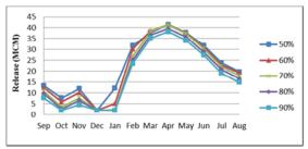
Figure5 Release from jarreh dam in different inflow percentage
