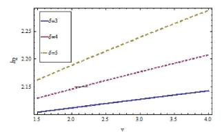
Figure 8: Thickness of the coated fiber optics versus ratio of the radii for different values of  $\delta$  at fixed values of  $\Lambda_1 = 4$ ,  $\Lambda_2 = 5$ ,  $\varepsilon_2 = 4$ ,  $\lambda_2 = 4$ ,  $\eta_2 = 7$ , v = 0.4,  $\Omega = 2$ ,  $h_1 = 0.06$ .
