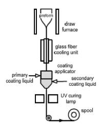
Figure 1: Double layer optical fiber coating in weton-wet coating process
