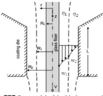
Figure 2: **PTT** flow model of double-layer coating in the secondary coating die
