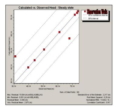
Figure 8: Results of the Steady State Calibration
