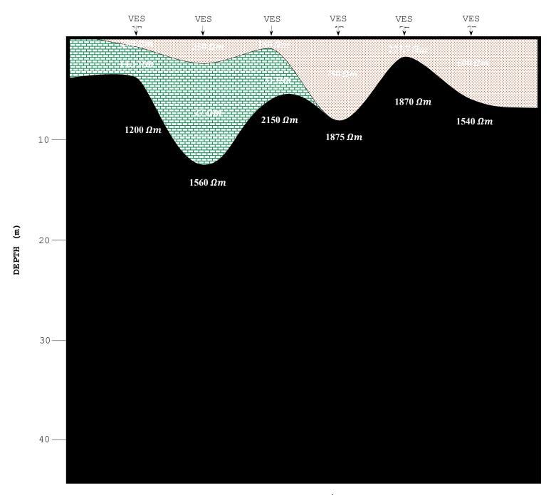
FIG. 4: Geoelectric section along profiles B-Bi
