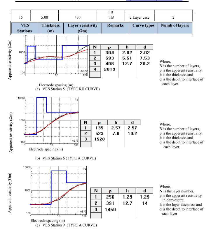
FIG. 2: Typical curve types and models obtained from the study area.
