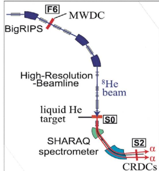
Figure 4: Shows The schematic of the experimental set up is based on three steps. Starting with the production of  $^8\text{He}$ , which then collides with  $^4\text{He}$  and the reaction products are then detected in the spectrometer [16].
