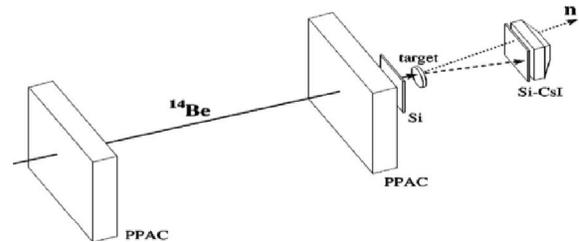
Figure 2: Shows the experimental setup of  $^{14}\text{Be} + ^{12}\text{C} \rightarrow ^{10}\text{Be} + 4n$  reaction. From left to right the beam tracking detectors, the ( $^{12}\text{C}$ ) target and a silicon detector for the detection of charged fragments ( $^{10}\text{Be}$ ) [12].
