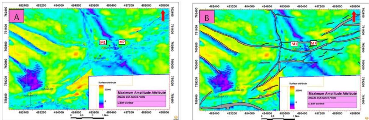
Figure 10 A) Maximum Amplitude Attribute Map On top U.BAH. B) Maximum Amplitude overlaid by interpreted Fault Polygons.
