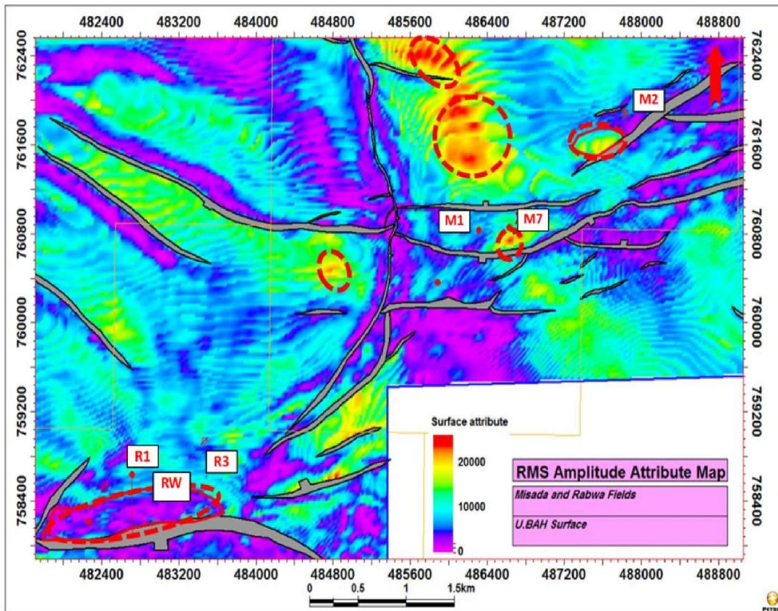
Figure 8 RMS. Amplitude Attribute Map overlaid by structure fault polygons
