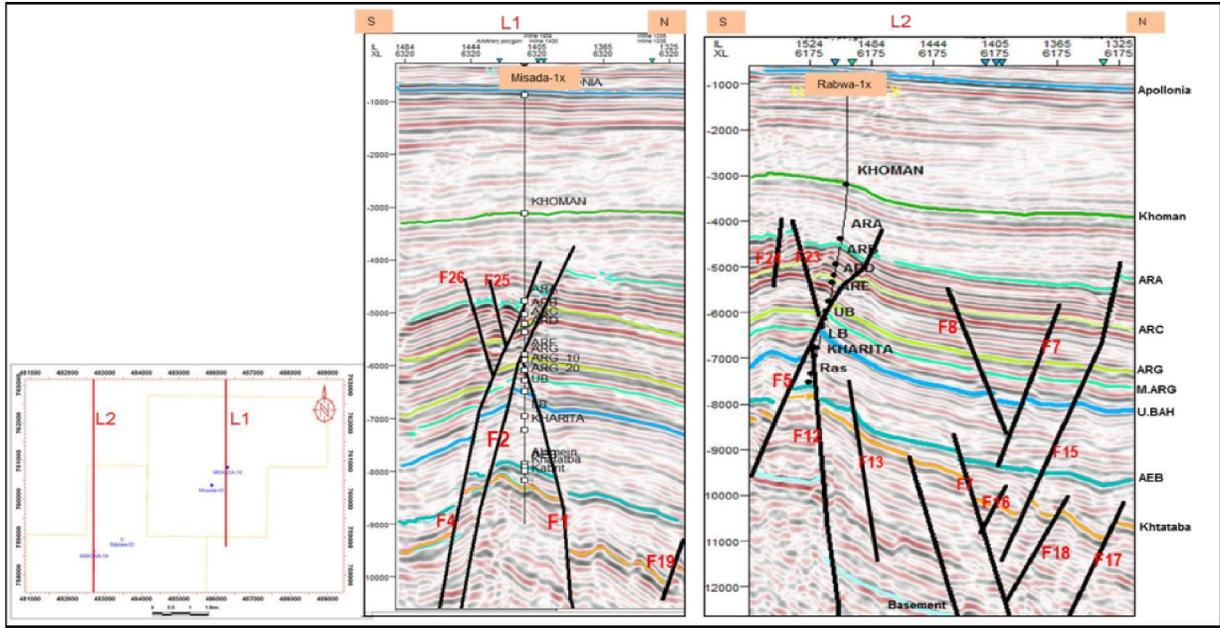
Figure 5 Two seismic cross sections showing the picked horizons and fault interpretation.
