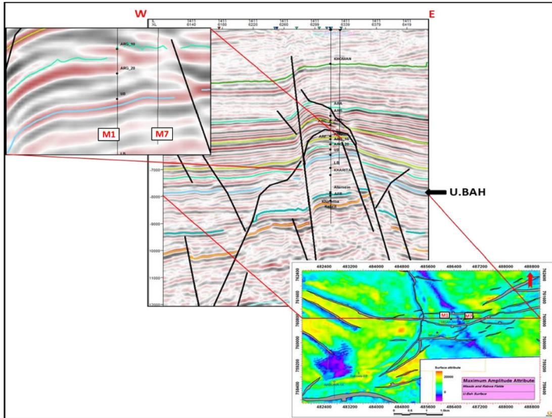
**Figure 11** E-W seismic line shows that the barrier between the wells M1 and M7 is not related to structure.
