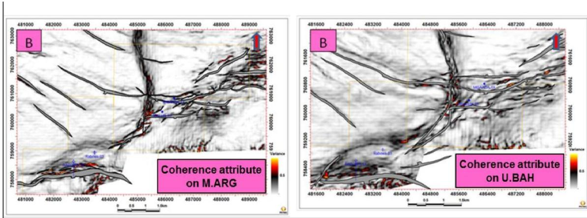
Figure 7 Coherence Attribute Maps for both M.ARG and U.BAH Horizons A) Coherence Attribute B) Coherence Attribute overlaid with fault polygons.
