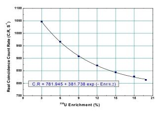
Figure 6. Calculated real coincidence count rate as a function of  $^{235}$ U enrichments ( $^{235}$ U mass is 100 g while the enrichment changes by changing the amount of  $^{238}$ U and  $^{234}$ U).
