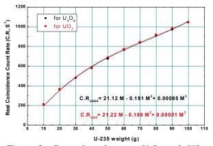
Figure 3. Comparison between  $U_3O_8$  and  $UO_2$  calculated real coincidence count rate for a wide range of <sup>235</sup>U masses.
