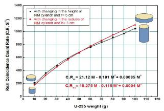
Figure 2. The calculated real coincidence count rate for a wide range of  $^{235}$ U masses content in  $U_3O_8$  in a cylindrical shape.
