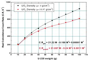
Figure 5. Calculated real coincidence count rate for a wide range of  $^{235}$ U mass content in UO<sub>2</sub> (3.0% enriched) with two different densities.
