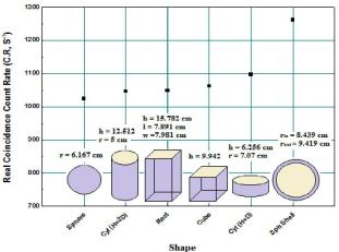
**Shape** Figure 7. The Calculated real coincidence count rate for 100 g of  $^{235}$ U content in U<sub>3</sub>O<sub>8</sub> (3.0% enriched) with density 4.0 g/cm<sup>3</sup> for different shapes
