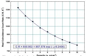
Figure 4. Calculated real concidence count rate for 100 g of  $^{235}$ U content in U<sub>3</sub>O<sub>8</sub> (3.0% enriched) as a function of density.
