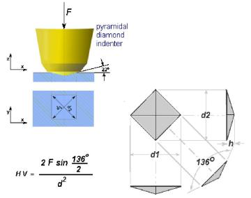
Fig. (2): Vickers hardness test scheme.
