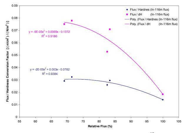
Fig.(6): Represent the stainless steel hardness to flux conversion constant based on the <sup>115</sup>In neutron flux.
