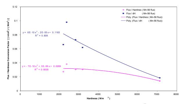
Fig.(7): Represent the stainless steel hardness to flux conversion constant based on the <sup>55</sup>Mn neutron flux.
