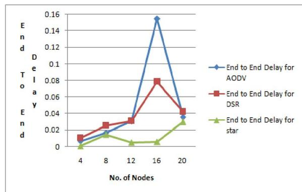
Fig. 4 End to End Delay Vs No. of Nodes for Packet sizes 256 bytes
