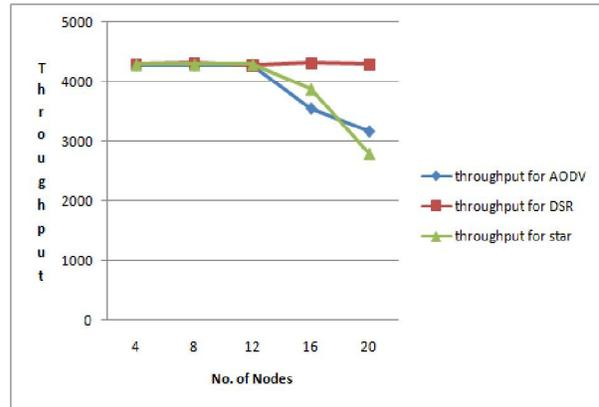
Fig.2 Throughput Vs No. of Nodes for Packet sizes 512 bytes
