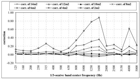
Fig.2c: absorption correction surface area for sponge material
