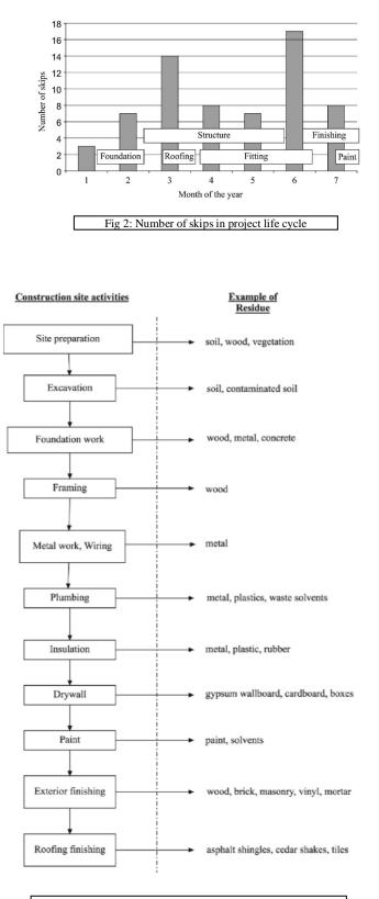
Fig 3: Construction works and material waste generated in that
