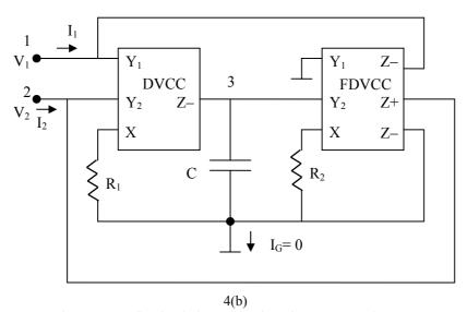
Figure 4 Two floating inductor circuits using DVCC and FDVCC [11]
