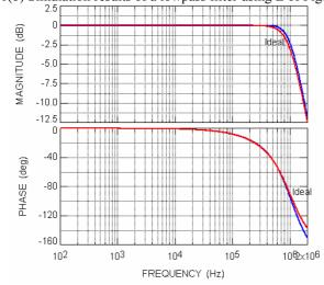
Fig 10(c) Simulation results of a lowpass filter using L of Figure 5
