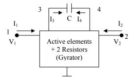
Figure 1(b) Generalized Type B configuration
