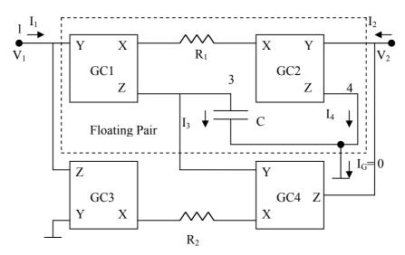
Figure 2. A floating inductor using four generalized conveyor
