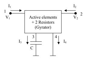
Figure 1(a) Generalized Type A configuration
