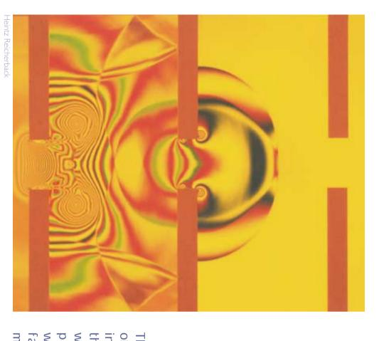
The colored picture demonstrates interference of a shock wave passing through a set of partitions in a two-dimensional flow in a shock tunnel. In the picture the portrait of a woman is revealed where her breast are, practically, vortices. In its passage through the partitions, the plane shock wave is transformed to cylinder creating the face. The eyes are, again, vortices where the mouth is equal density lines
