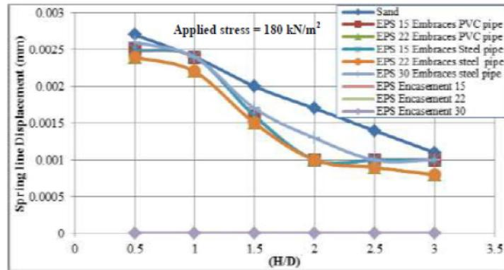
Figure 11. Spring line displacement in case of embedded EPS block Encasement and Embraces upper PVC and Steel pipe model with relative EPS densities and (H/D).
