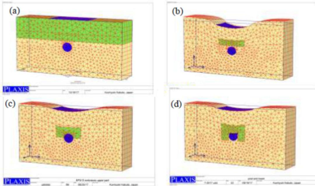
Figure 3. Numerical model in case of EPS block (a) Embankment (b) Imperfect ditch method (c) Embraces upper pipe (d) Encasement pipe.
