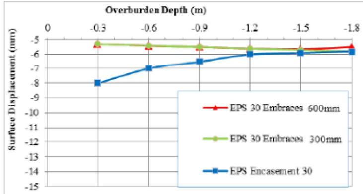
Figure18. Surface displacement subjected to surface stress 180 kN/m<sup>2</sup> in case of EPS30 models on 600 mm
