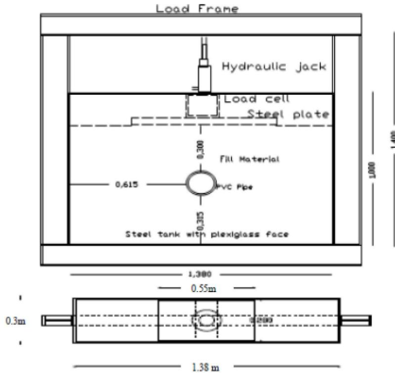
Figure 1. The loading frame and steel tank
