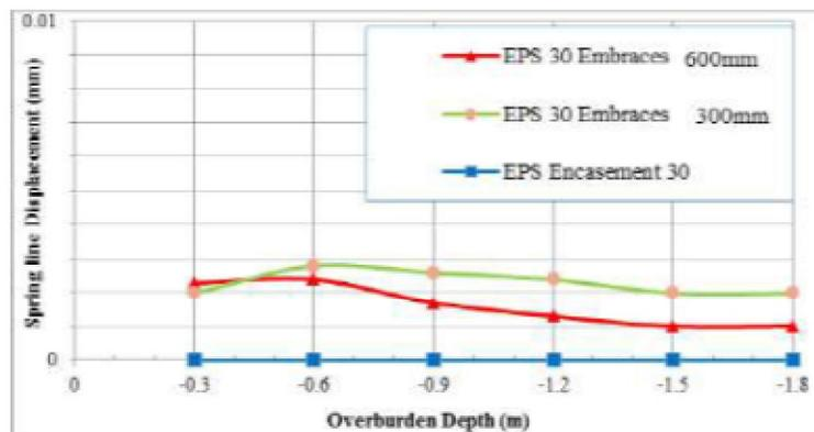
Figure 20. Spring line displacement subjected to surface stress 180kN/m<sup>2</sup> in case of EPS 30 models on 600 mm (24”) and 300 mm (12”) pipes.
