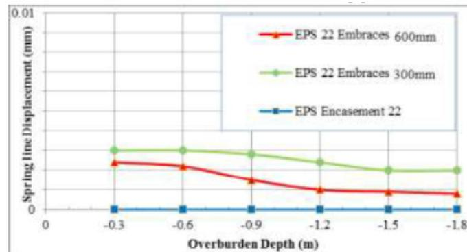
Figure17. Spring line displacement subjected to surface stress 180 kN/m<sup>2</sup> in case of EPS 22 models 600 mm (24”) and 300 mm (12”) pipes
