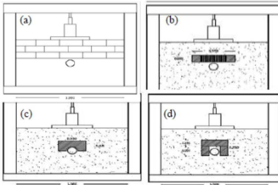
Figure 2. The experimental model (a) Embankment (b) Imperfect ditch method (c) Embraces upper pipe (d) Encasement pipe
