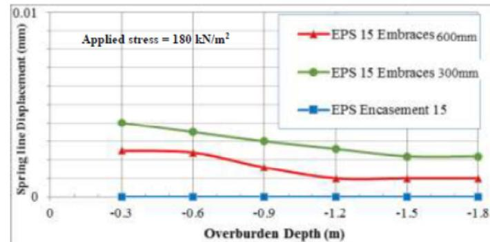
Figure 14. Spring line displacement in case of EPS 15 models 600 mm (24'') and 300 mm (12'') pipes
