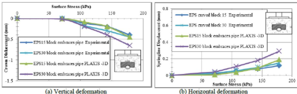
Figure 5. Deformation of UPVC buried pipe in case of embedded EPS block embraces the Pipe upper part model.
