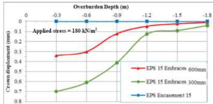
Figure 13. Crown displacement in case of EPS 15 models on 600 mm (24'') and 300 mm (12'') pipes
