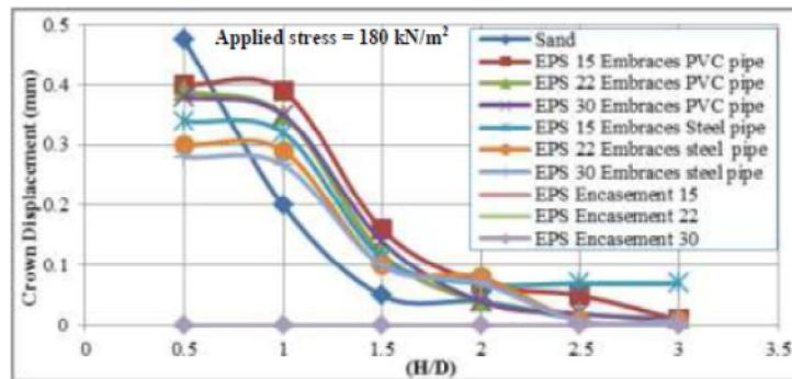
Figure 10. Crown displacement in case of embedded EPS block Encasement and Embraces upper PVC and Steel pipe model with relative EPS densities and (H/D).
