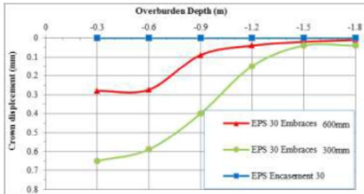
Figure19. Crown displacement subjected to surface stress 180kN/m<sup>2</sup> in case of EPS 30 models on 600 mm (24”) and 300 mm (12”) pipes.
