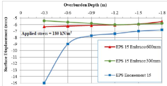
Figure 12. Surface displacement in case of EPS 15 models on 600 mm (24'') and 300 mm (12'') pipes
