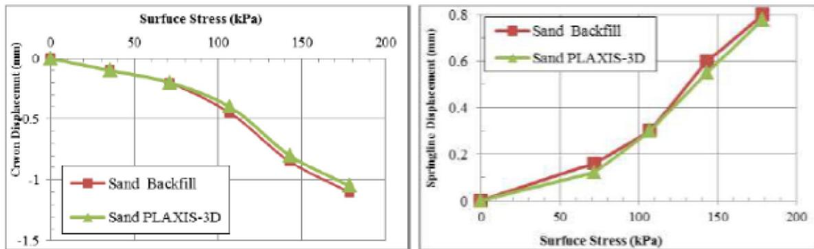
Figure 4. Deformation of UPVC buried pipe in case of sand back-fill model
