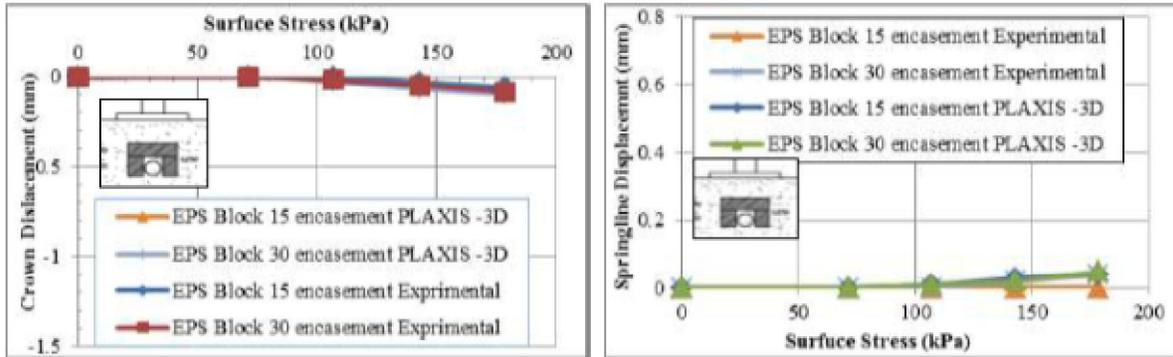
Figure7. Deformation of UPVC buried pipe in case of embedded EPS encasement blocks model.
