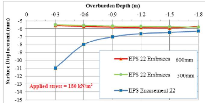
Figure 15. Surface displacement subjected to surface stress 180 kN/m<sup>2</sup> in case of EPS 22 models on 600 mm (24”) and 300 mm (12”) pipes
