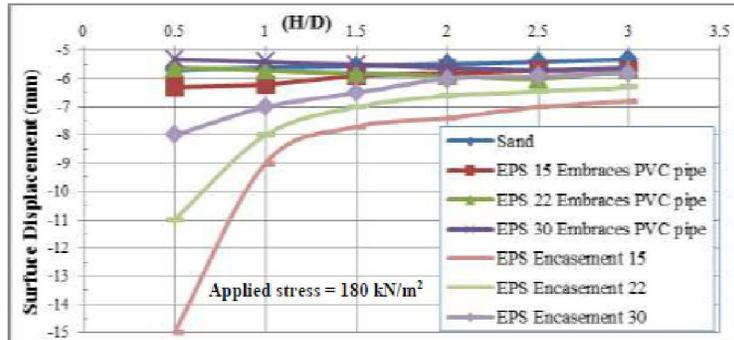
Figure (9) Surface displacement in case of embedded EPS block Encasement and Embraces upper PVC and Steel pipe model with relative EPS densities and (H/D).
