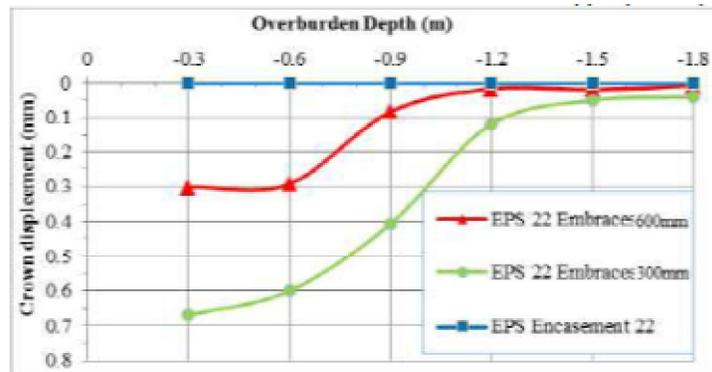
Figure 16. Crown displacement subjected to surface stress 180 kN/m<sup>2</sup> in case of EPS 22 models on 600 mm (24”) and 300 mm (12”) pipes
