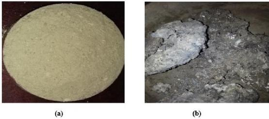
Fig. 6: (a) Zeolite, (b) Red-Mud (Aluminum slag) as
