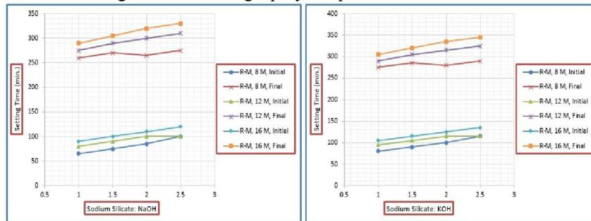
**Fig. 13:** Effect of the NaOH molarity with different Na<sub>2</sub>SiO<sub>3</sub>/NaOH ratios and KOH molarity with different Na<sub>2</sub>SiO<sub>3</sub>/KOH ratios on the setting time of Red-Mud geopolymer pastes.
