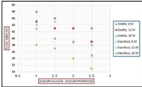
Fig. 9: Effect of the NaOH molarity with different Na<sub>2</sub>SiO<sub>3</sub>/NaOH ratios on flowability
