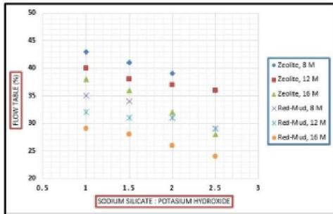
Fig. 10: Effect of the KOH molarity with different Na<sub>2</sub>SiO<sub>3</sub>/KOH ratios on flowability
