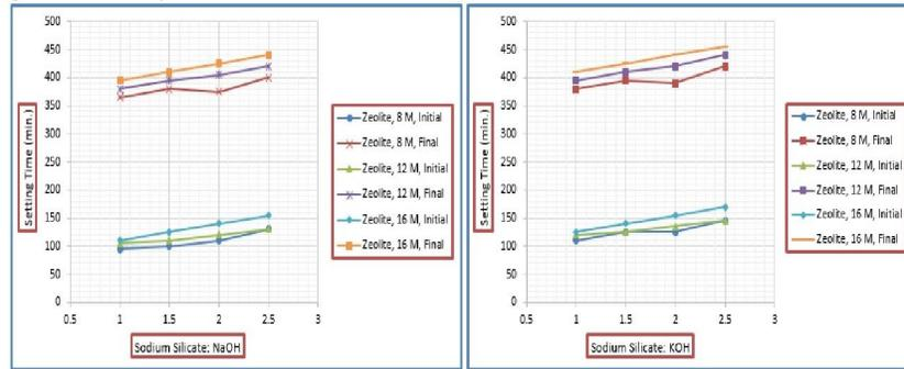
**Fig. 12:** Effect of the NaOH molarity with different Na<sub>2</sub>SiO<sub>3</sub>/NaOH ratios and KOH molarity with different Na<sub>2</sub>SiO<sub>3</sub>/KOH ratios on the setting time of zeolite geopolymer pastes.
