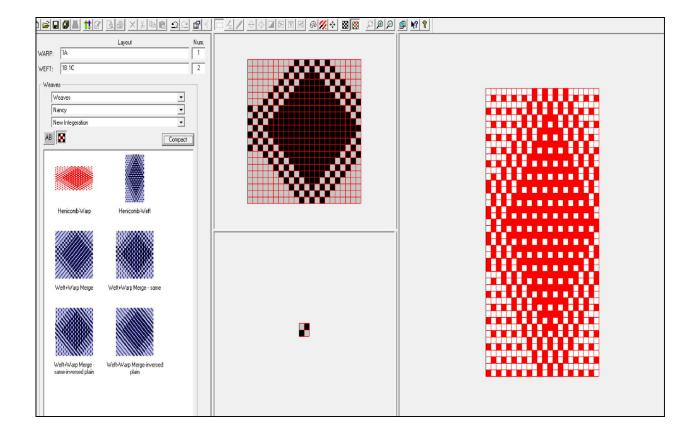
**3** - The integration 1:1 by weft and 1:1 by warp with Extrusive repetition of weft movement. If the plain weave 1/1 is symbolized by, the symbol (A) and honeycomb weave symbol (b). Then the integration will be as (AA: BB).
