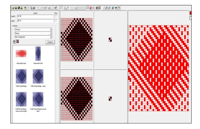
6 - The integration 1:1 by weft and 1:1 by warp with reversed repetition of weft movement and exchange the plain weave in the second repetition.
