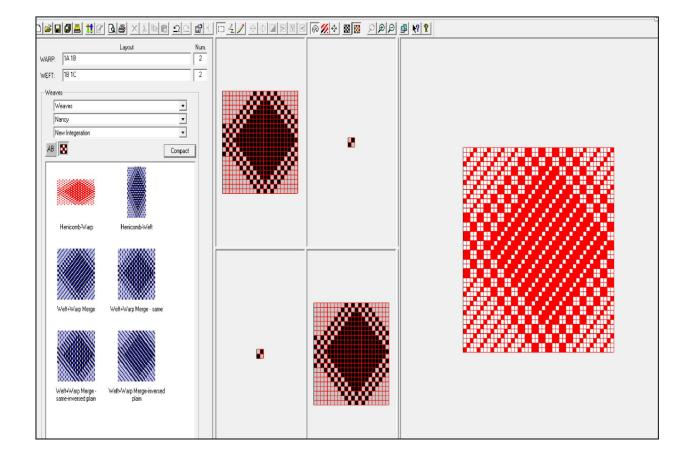
5 - The integration 1:1 by weft and 1:1 by warp with Extrusive repetition of weft movement and reverse the plain weave 1/1 in the second repetition.
