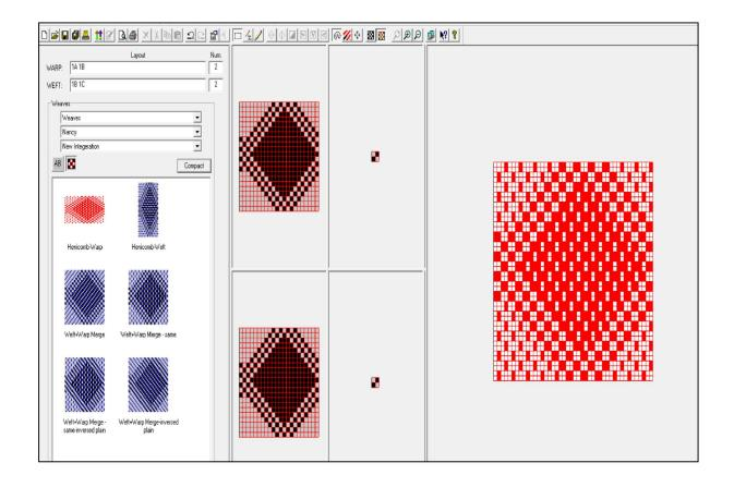
**4** - The integration 1:1 by weft and 1:1 by warp with reversed repetition of weft movement. If the plain weave 1/1 is symbolized by, the symbol (A) and honeycomb weave symbol (b). Then the integration will be as (BA: AB).
