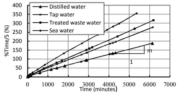
**Fig.4:** Time/S ratio versus time for different water types (Using Proctor cylinder)
