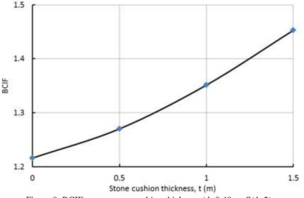
Figure 9. BCIF versus stone cushion thickness (d=0.40 m, S/d=2)
