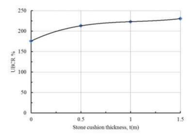
Figure 8. UBCR versus different values of stone cushion thickness (d=0.40 m, S/d=2)
