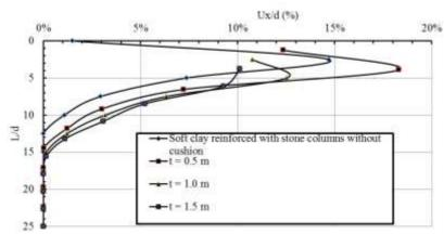
Figure 13. Lateral displacement to diameter ratio  $(U_x/d)$  versus L/d for various values of stone cushion thickness (t) (d=0.4 m, S/d=2)
