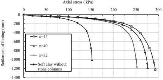
Figure 2a. Axial stress versus settlement for various values of  $\varphi$  (d = 0.40 m, L/d=10, S/d=2.0)
