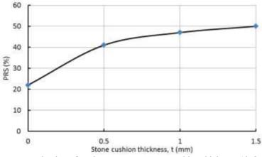
Fig. 10. Percentage reduction of settlement versus stone cushion thickness (d=0.40 m, S/d=2)
