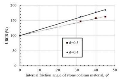
Figure 3. UBCR versus internal friction angle of stone material
