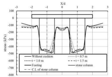
Figure 11. Contact stress distribution for various values of stone cushion thickness (t) (d=0.4m, S/d=2.0)
