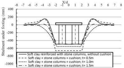
Figure 12. Vertical settlement dist ribution beneath the footing for various values of stone cushion thickness (t) (d=0.4 m, S/d=2)
