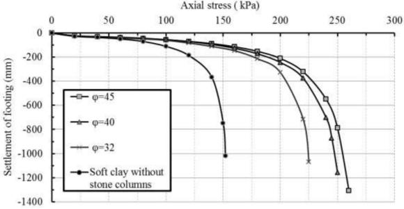
Figure 2b. Axial stress versus settlement for various values of  $\varphi$  (d = 0.50 m, L/d=10, S/d=2)
