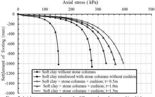
Figure 7. Axial stress versus settlement for different values of stone cushion thickness (d=0.40 m, S/d=2)
