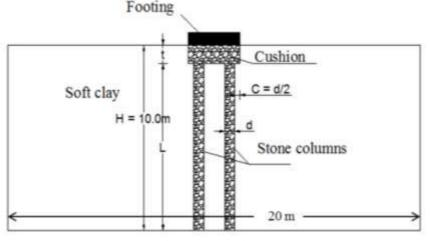
Figure 1. Model geometry
