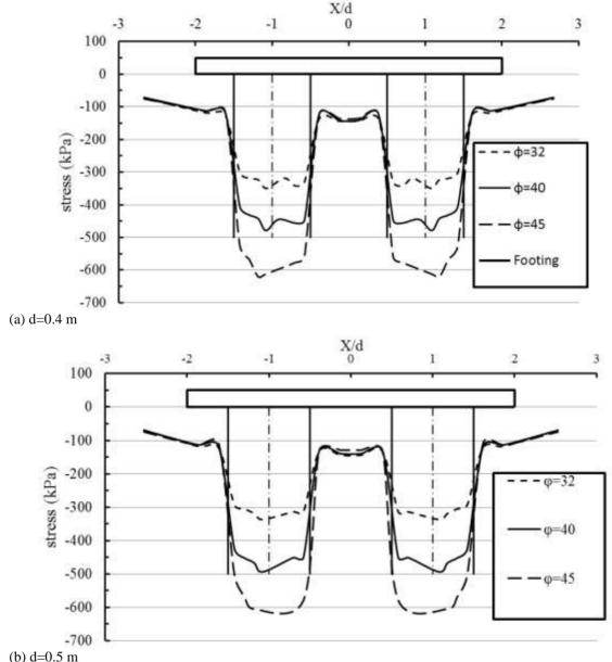
Figure 4 Contact stress distribution for various values of angle of internal friction of stone ( $\phi$ ) (L/d=10, S/d=2.0]
