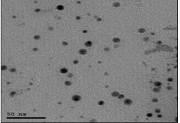
*Figure (5):* TEM image of silver nanoparticles (50 nm scale).
