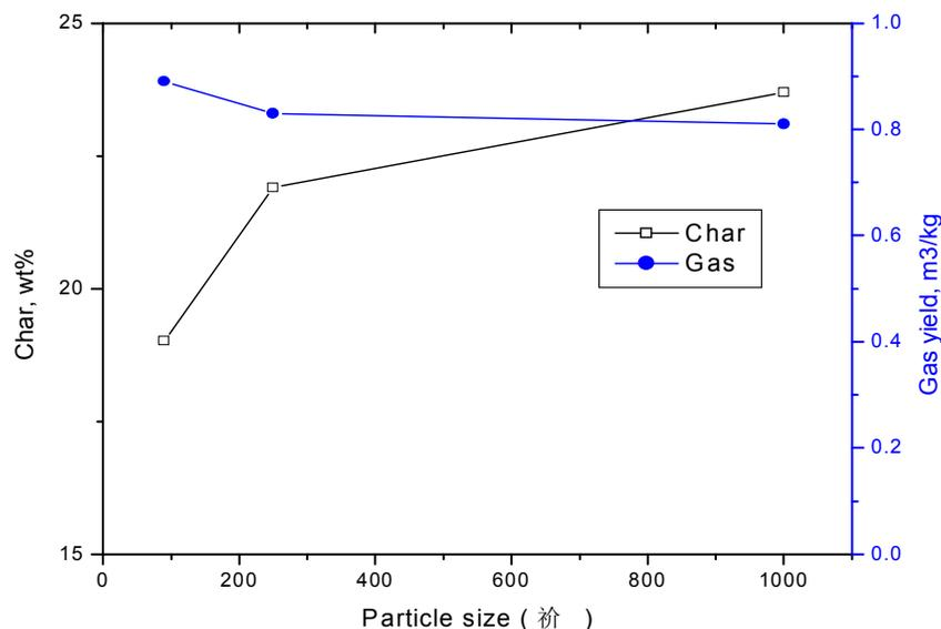
Figure 7. Effect of particle size on gasification processes
