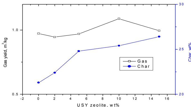
Figure 11. Effect of USY zeolite on the gasification processes ER: 0.25, Temp. 800°C, Time of reaction: 90 min
