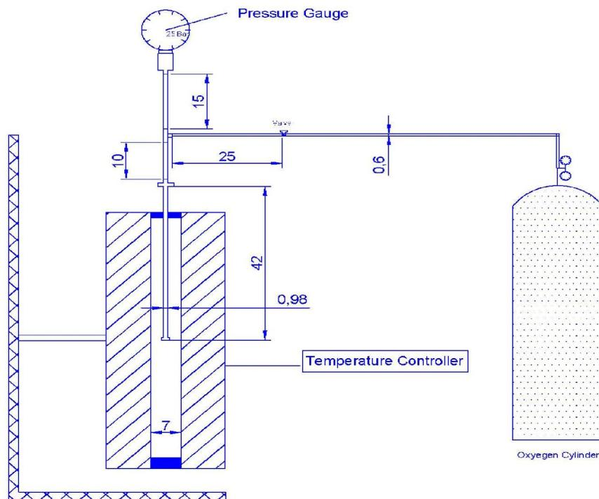
Figure 2. Reactor for gasification of saw dust (Dimensions in cm)
