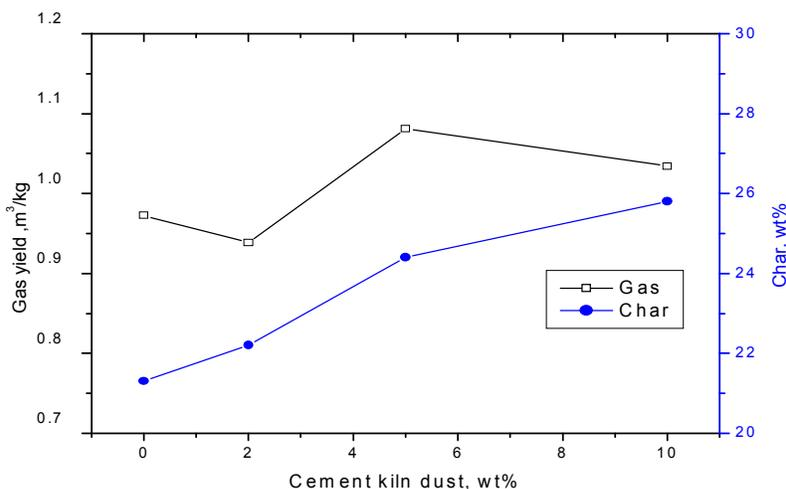
Figure 12. Effect of cement kiln dust on the gasification processes
