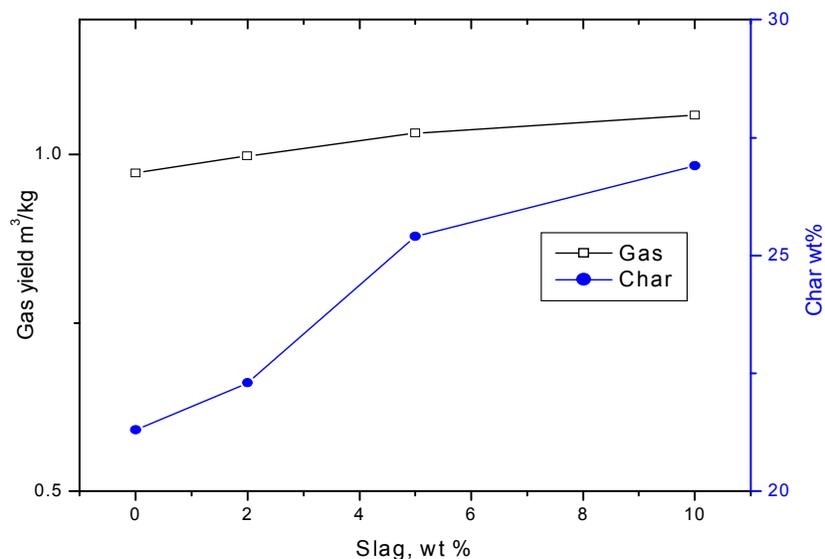
Figure 10. Effect of granulated slag on the gasification processes
