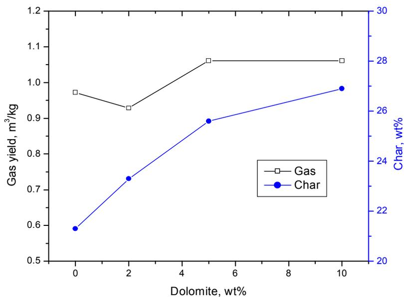
Figure 14. Effect of dolomite catalyst on gasification of saw dust
