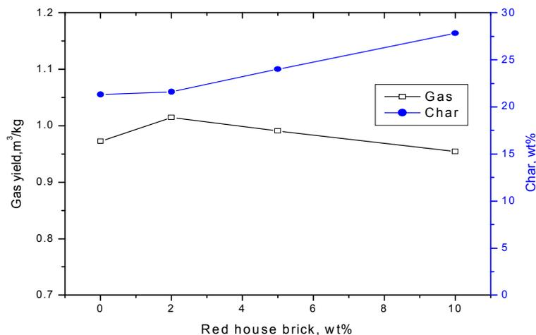
Figure 13. Effect of red house brick on the gasification processes
