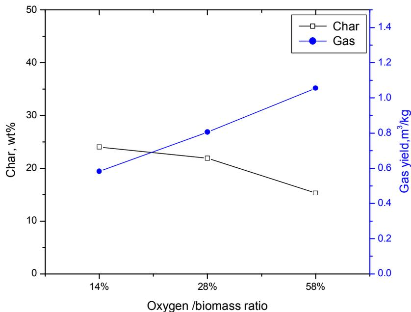
Figure 4. Effect of Oxygen/biomass equivalence ratio on gasification products
