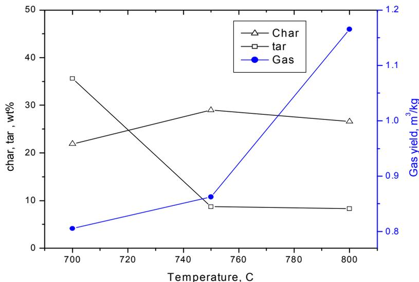
Figure 5. Effect of temperature on gasification products
