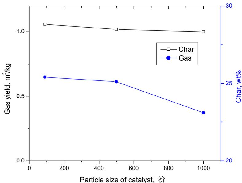
Figure 8. Effect of particle size of catalyst on gasification processes
