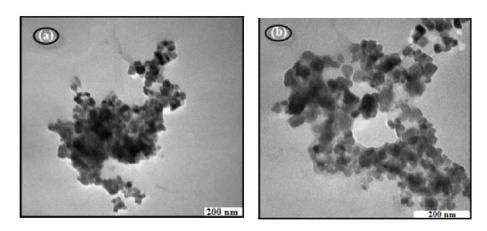
Figure 7. TEM images (a) Fe<sub>3</sub>O<sub>4</sub> nanoparticles and (b) PAMAM dendrimer-coated iron oxide nanoparticles at direct magnification 50000X.
