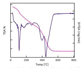
**Figure 4.** TGA/DrTGA curves of PAMAM dendrimer – coated iron oxide.
