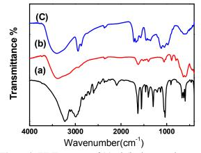
Figure 2. FT-IR spectra of (a) tris(hydroxymeth -yl )amino methane hydrochloride, (b) pure  $Fe_3O_4$  nanoparticles, and (c) PAMAM dendrimer – coated iron oxide.
