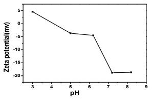
**Figure 6.** Zeta potential of PAMAM dendrimer coated–Fe<sub>3</sub>O<sub>4</sub> nanoparticles at different pH values.
