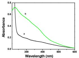
**Figure 5.** UV-Vis absorption spectra of  $Fe_3O_4$  (a) and PAMAM dendrimer–coated iron oxide (b).
