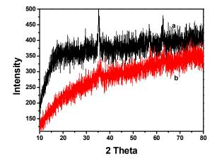
Figure 3. XRD patterns of (a)  $Fe_3O_4$ , and (b) and PAMAM dendrimer – coated iron oxide.
