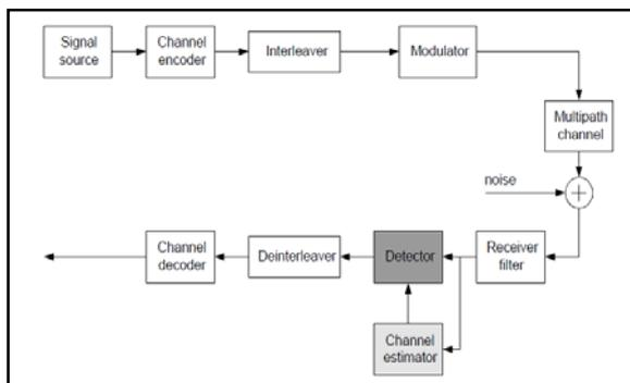
Figure [1]: layout block diagram for TDMA
