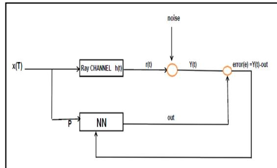
Figure [4]: block diagram for channel estimation using NN
