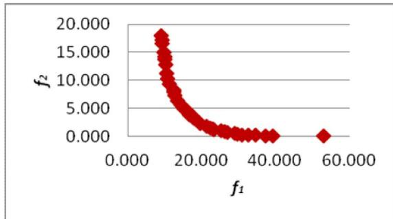
Figure 4. Set of 36 Pareto optimal solutions generated after the first iteration for the  $f_2$  objective
