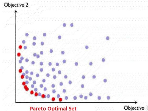
Figure 1. Two-objective space assuming the two objectives are to be minimized. The red points represent the Pareto frontier
