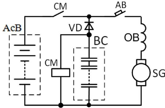
**Figure 1. Simplified start circuit of the starter of the locomotive TEM-2 electro-engine**
