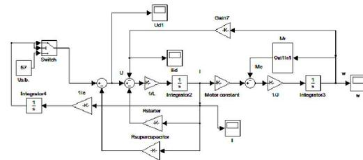
**Figure 2. A simulation model of a two-steps start process of the diesel shunting locomotive TEM-2**
