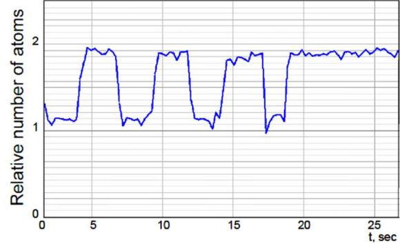
Fig.4. Plot of the number of MOT atoms in time. This plot was obtained from the state-of-the-art software for mentioned above digital camera Hamamatsu. It is clearly seen that detuning of the blue repumper laser from transition resonance and mechanical shutting lead to decreasing of the number of atoms down to initial value
