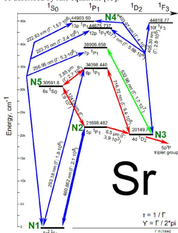
**Fig.1. Wavelength and decay rates of the  $^{87}\text{Sr}$  working transitions**
