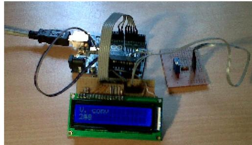
Figure 26. Visualization with LCD of data captured by the CAD.
