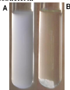
Fig. 1. A photograph showing Koline clay particles flocculated with Nocardioptis aegyptia culture filtrate(B) and control without biofloculant(A).
