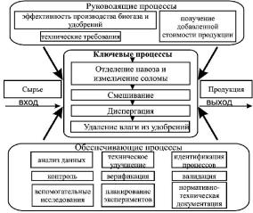
Figure 1 – Flow-process diagram of biogas unit
