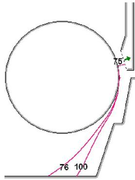
**Fig. 8. Paths of dust particles having the density of 1000 kg/m<sup>3</sup> when a cylinder is rotating at linear velocity  $v_{rot} = 0.5$  m/s and  $v_0 = 2$  m/s**
