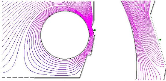
**Fig. 11. Flow lines for a cylinder rotating at linear velocity  $v_{rot} = 0.5$  m/s and  $v_0 = 1$  m/s**
