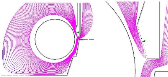
**Fig. 3. Flow lines for a cylinder rotating at linear velocity  $v_{rot} = 0.5$  m/s and  $v_0 = 0.5$  m/s**
