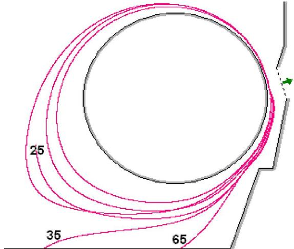
**Fig. 12. Paths of dust particles having the density of  $1000 \text{ kg/m}^3$  when the cylinder is rotating at linear velocity  $v_{rot} = 0.5$  m/s and  $v_0 = 1$  m/s**
