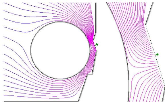
**Fig. 10. Flow lines for a resting cylinder and suction velocity  $v_0 = 1$  m/s**
