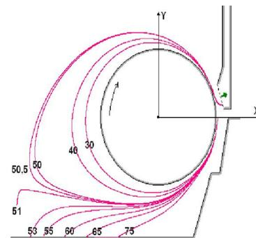
**Fig. 7. Paths of dust particles having the density of  $1000 \text{ kg/m}^3$  when a cylinder is rotating at linear velocity  $v_{rot} = 0.5$  m/s and  $v_0 = 1$  m/s**
