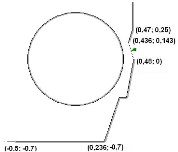
**Fig. 9. The flow pattern induced at a local exhaust by a roll-turning machine without air inflow between the local exhaust and the support**
