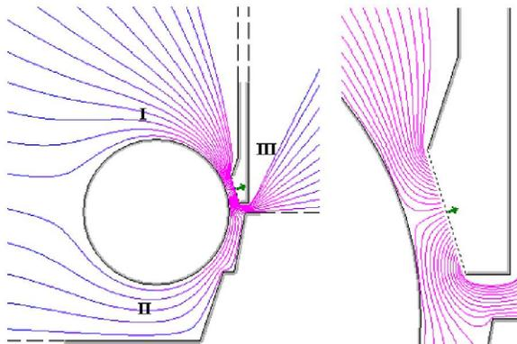
**Fig. 2. Flow lines for a resting cylinder and velocity  $v_0 = 2$  m/s**
