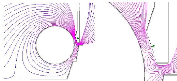
**Fig. 5. Flow lines for a cylinder rotating at linear velocity  $v_{rot} = 0.5$  m/s and  $v_0 = 2$  m/s**
