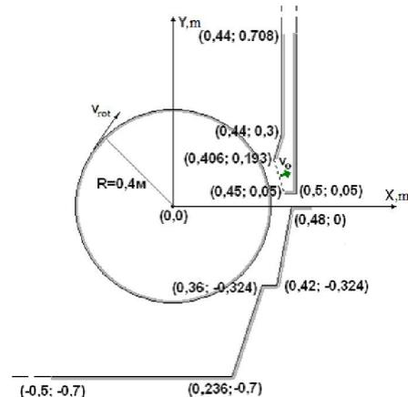
**Fig. 1. The flow pattern induced at a local exhaust by a roll-turning machine**
