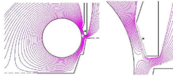
**Fig. 4. Flow lines for a cylinder rotating at linear velocity  $v_{rot} = 0.5$  m/s and  $v_0 = 1$  m/s**
