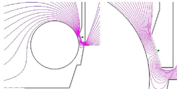
**Fig. 6. Flow lines for a cylinder rotating at linear velocity  $v_{rot} = 0.5$  m/s and  $v_0 = 4$  m/s**
