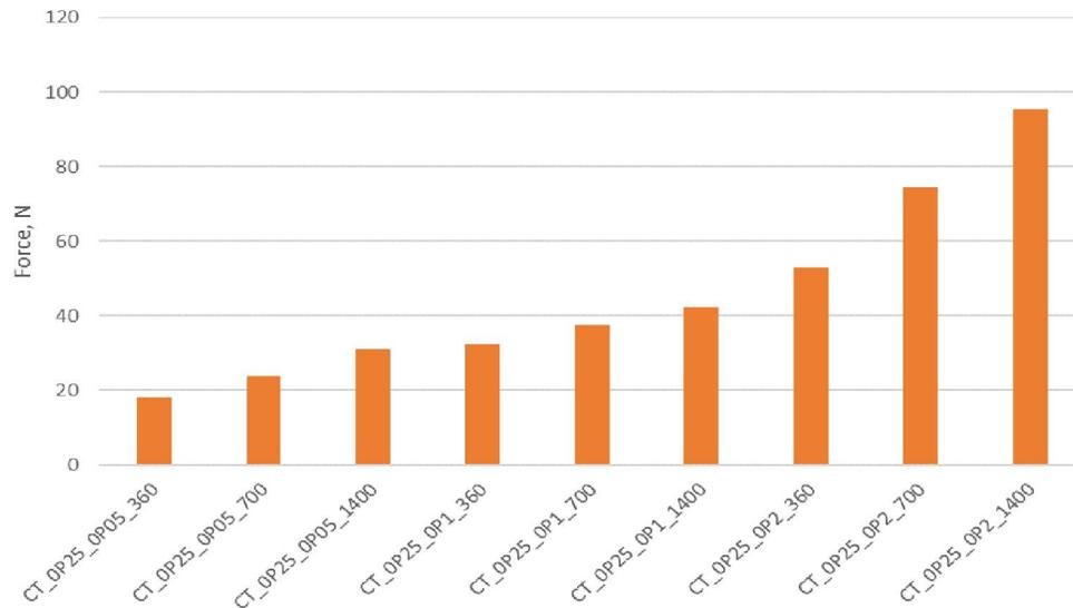
Figure 5: Machining forces as recorded by the force dynamometer for  $d = 0.25 \text{ mm}$
