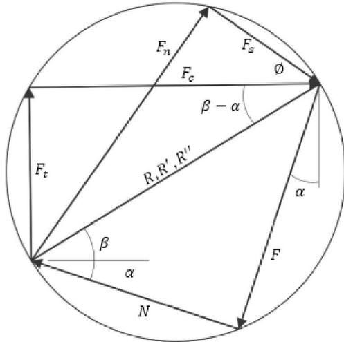
Figure 3: Mohr's circle for linking various types of machining forces (after (Groover 2010))
