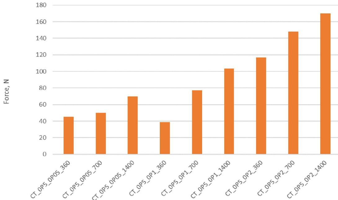
Figure 6: Machining forces as recorded by the force dynamometer for  $d = 0.5 \text{ mm}$
