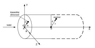
Fig. 1. Location of the ultrasound transmitter and receiver inside the pipe
