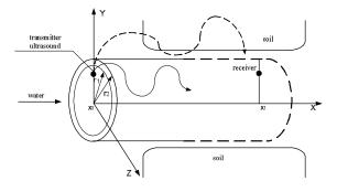
Fig. 2. Ultrasound extending inside an underground pipe
