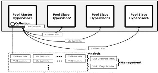
Figure 3. VM Lifecycle Tracing Program Flow
