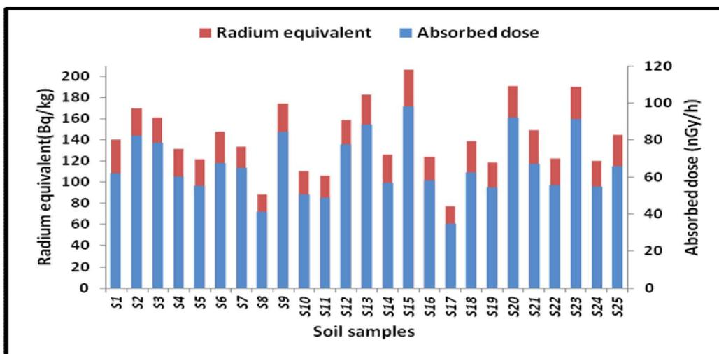
Fig.3 Absorbed dose rate (nGy/h) Radium equivalent (Bq/Kg) for soil samples from different locations in Industrial Yanbu city, Saudi Arabia.
