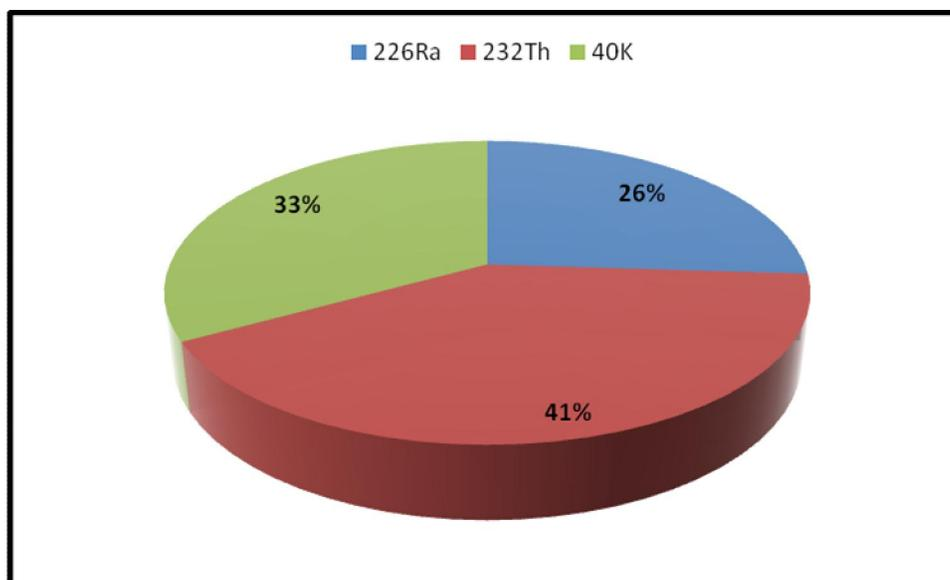
Fig. 4 Percentage contribution to the total absorbed dose of  $^{226}\text{Ra}$ ,  $^{232}\text{Th}$  and  $^{40}\text{K}$
