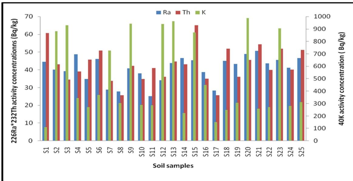
Fig.2 Activity concentrations of  $^{226}\text{Ra}$ ,  $^{232}\text{Th}$  and  $^{40}\text{K}$  for surface soil samples collected from different locations of the Industrial Yanbou city, Saudi Arabia
