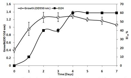
Figure 3. Growth and emulsification index of *Bacillus* sp. E34, grown at 37°C with shaking at 160 rpm with glucose as a carbon source.
