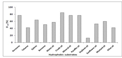
Figure 8. Emulsification index (EI<sub>24</sub> %) of *Bacillus* sp. E34 biosurfactant produced in the optimized medium against some hydrophobic substrates.
