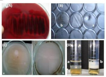
**Figure 1.** (A) Haemolytic activity of E34 strain on blood agar within 24 h of incubation at room temperature. (B) Drop collapse test: (a) Unculture media (control), not collapsed. (b) E34 supernatant on the oily surface, collapsed. (C) Oil displacment test: (a) Culture media alone (control) (b) the spreading of E34 biosurfactant on oil surface layer. (D) Emulsification index test: (a) Uncultured LB medium (b) Emulsion formation of E34 biosurfactant.
