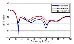
Figure 3. The return loss of the proposed UWB slot antenna at B=12mm, Ws=18mm, and different values of the triangular stub height (H).
