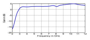
Figure 6. The gain of the proposed antenna as a function of
