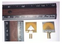
Figure 7.The prototype of the proposed UWB slot antenna.
