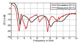
Figure 8. The simulated and measured return loss of the proposed UWB slot antenna.
