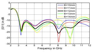
Figure 2. The return loss of the proposed UWB slot antenna at H=9.5mm, Ws=18mm, and different values of the triangular stub base (B).
