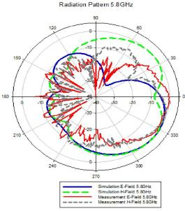
Figure 10. Simulated and Measured Radiation Pattern at 5.8 GHz.
