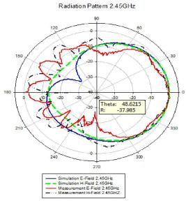
Figure 9. Simulated and Measured Radiation Pattern at 2.45 GHz.
