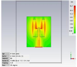
Figure 6. Current distribution at H-Field at 2.45 GHz
