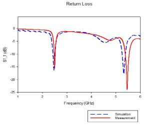
Figure 8. Simulated and Measured Return Loss
