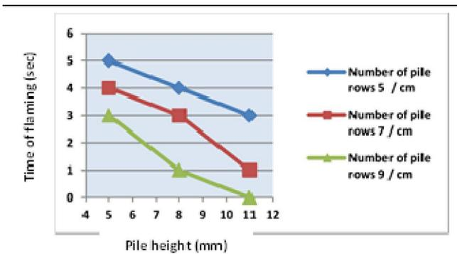
Figure (11): Effect of pile height and number of pile rows / cm for samples made of pile yarn material polypropylene /Acrylic 60/40% on time of flaming
