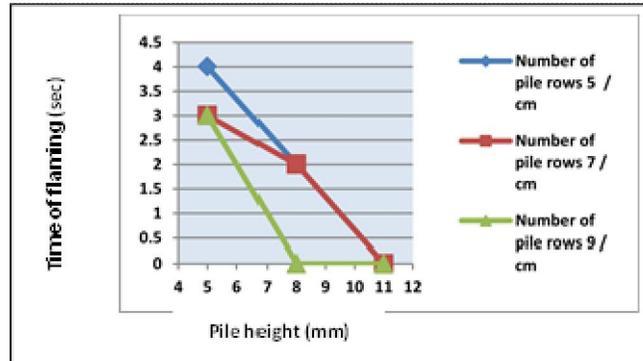
Figure (10): Effect of pile height and number of pile rows / cm for samples made of pile yarn material polypropylene 100% on time of flaming
