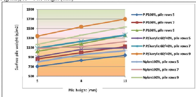
Figure [1]: Effect of pile yarn material, number of pile rows, and pile height on surface pile weight of carpet.
