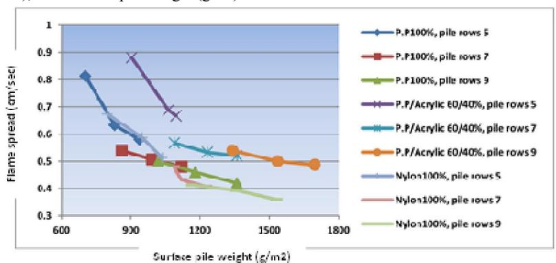
Figure (5): Effect of pile yarn material, number of pile rows, and surface pile weight on flame spread of carpet surface pile (cm/sec).
