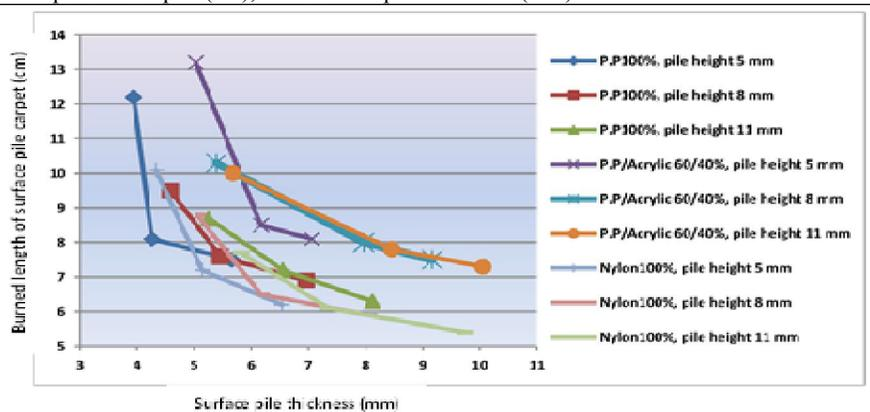
Figure (4): Effect of pile yarn material, pile height, and surface pile thickness on burned length of carpet surface pile (cm).
