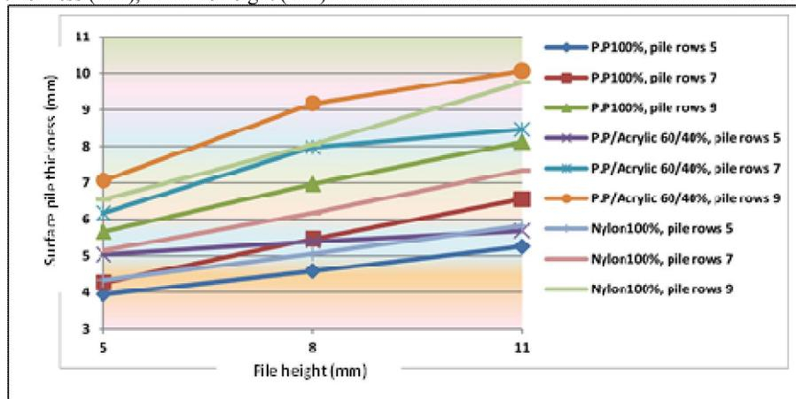
Figure (2): Effect of pile yarn material, number of pile rows, and pile height on surface pile thickness of carpet.
