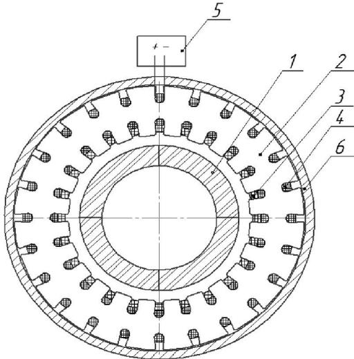
**Figure 1: General view of non-contact magneto-electric generator according to patent illustrating where 1 is the rotor, 2 is the stator, 3 is the slot winding, 4 is the toroidal winding, 5 electrically-connected to DC power supply where stator is pressed into the ferromagnetic cylinder (6) with saturation flux density which is equal to the saturation induction of stator or exceeds it.**
