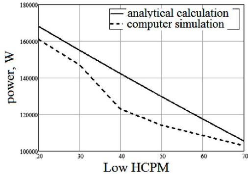
**Figure 2: Dependence of capacity of the generator with the high-coercivity permanent magnets on the temperature of the permanent magnets.**
