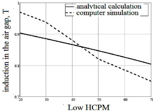
**Figure 3: Dependence of the air gap induction of the generator with the high-coercivity permanent magnets on the temperature of the permanent magnet.**
