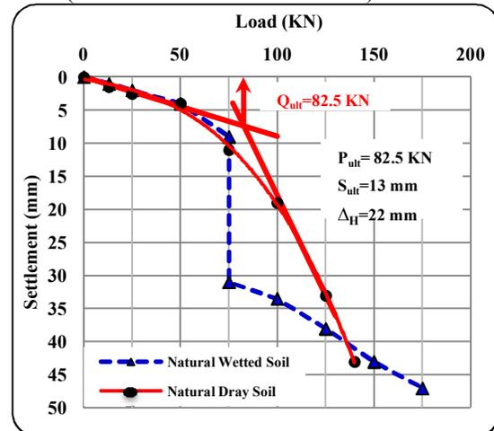
Figure 6. Load-settlement response for plate tests on natural and wetted soil.
