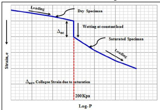
**Figure 2. Schematic diagram of single oedometer collapse test.**
