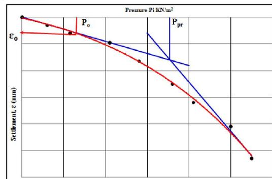
**Figure 4. Diagram illustrating load intensity-bearing plate settlement curve.**
