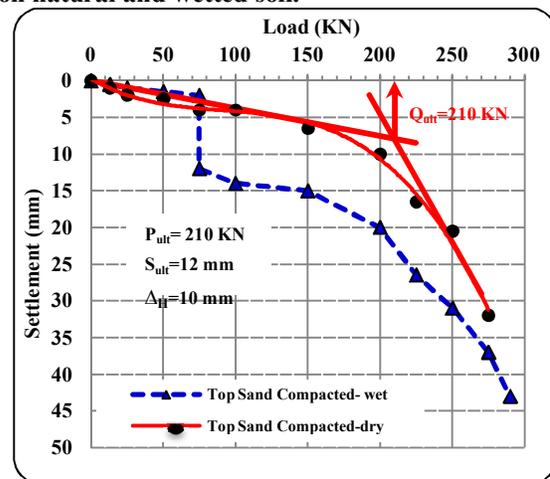
Figure 7. Load-settlement response for plate tests on top sand compacted and compacted wetted.
