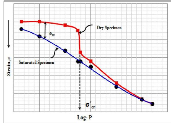
**Figure 3. Schematic diagram of double oedometer test.**
