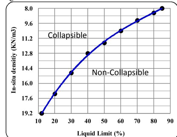
Figure 1. Identification of collapsible plastic soils
