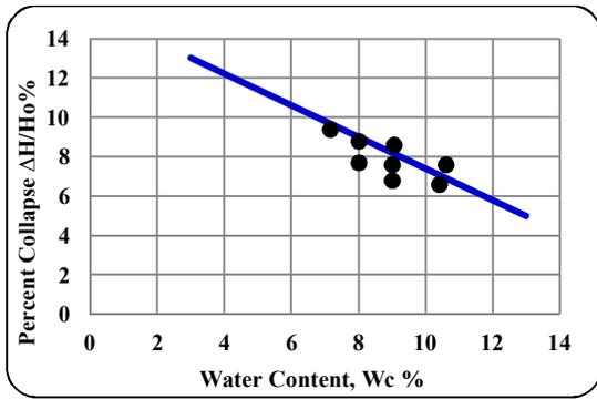
Figure 5. Effect of the initial water content, dry density on the amount of collapse
