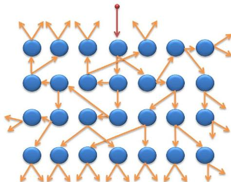
Fig. 1 Branched chain reaction branching parameter  $\bar{U} = 2$ .
