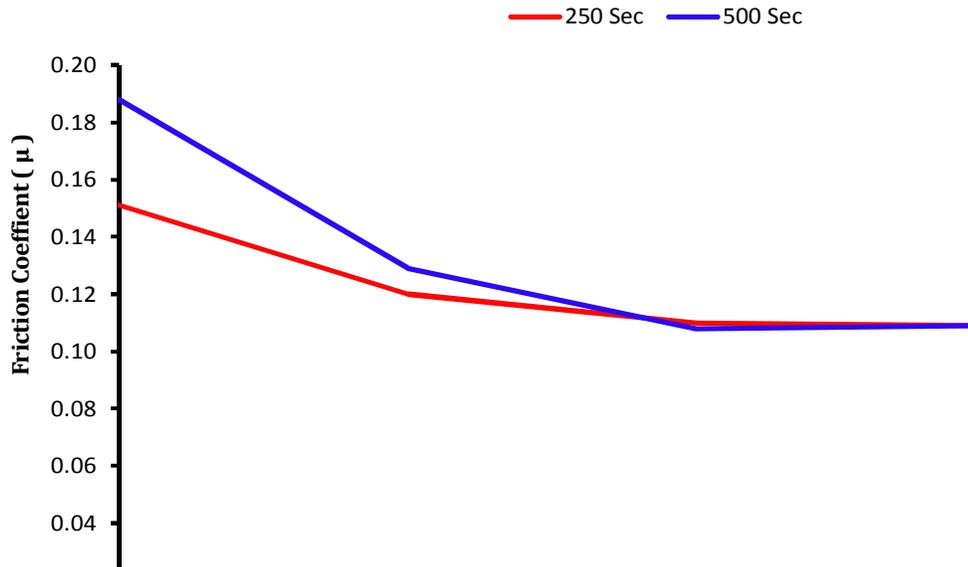
Figure 6: Coefficient of friction against sliding speed at a constant applied load (101 N).
