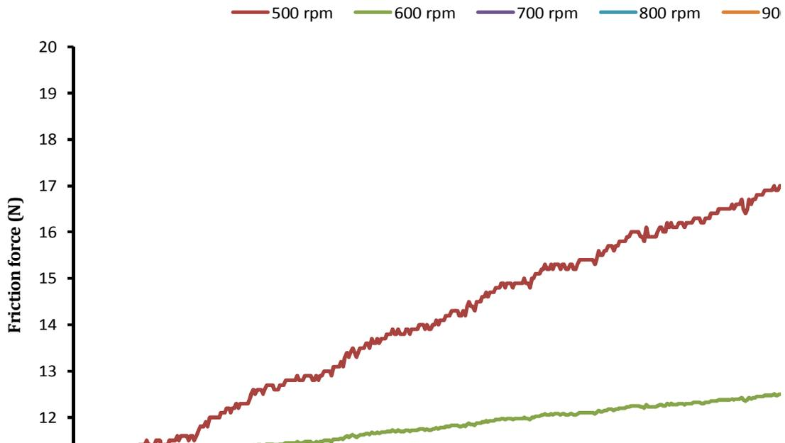
Figure 5: Friction force as a function of running time under a constant applied load of 101N.
