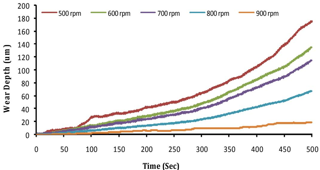
Figure 3: Variation of wear depth - running time at different sliding speeds (constant applied load 101 N)
