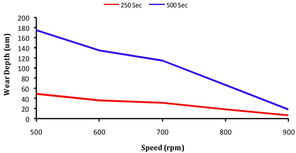
Figure 4 Effect of speed on wear depth (µm) at a constant applied load (101 N)
