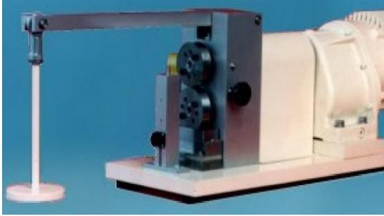
Figure 1: Block-on-ring machine
