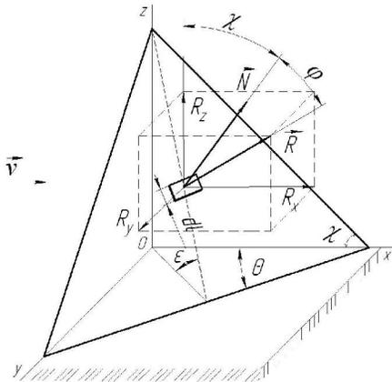
Figure 2 - Forces acting on a triangular wedge
